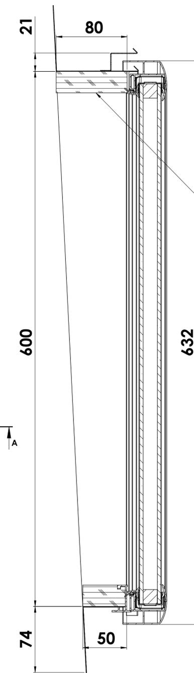
**profil rupture pont
